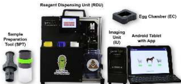
Fig. 1 Components of the automated system. The system consists of a reusable Sample Preparation Tool (SPT), which itself consists of a silicone bottle, a handle for sample homogenization and a dispensing tip with integrated filter; dispensable egg Chambers (EC) in which samples to be chemically treated and imaged; a Reagent Dispensing Unit (RDU); an Imaging Unit (IU); and an Android tablet with an App for capturing images from the IU and for turning eggs in the images.
